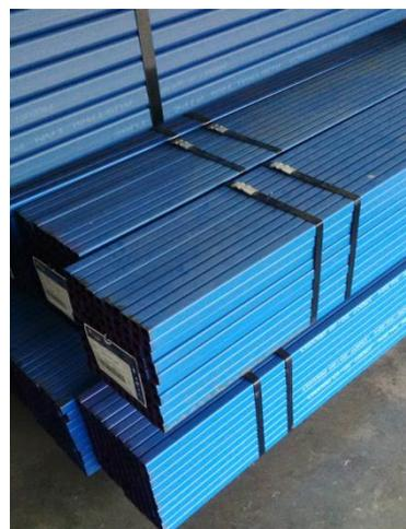
All kinds of Black round and hollow sections, galvanized and pre-galvanized pipes can be colour coated.
