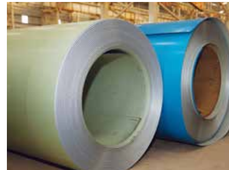
Implementation of India's first Thicker Colour Coating Line, offering superior coating thickness ranging from 1.60mm to 2.50mm
